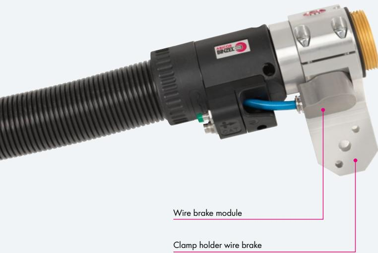
For tactile component search using the established ABIROB® W cable assembly, cable assemblies can now come with an optional wire clamp function to fix the wire. This function enables fixing of the wire in the cable assembly by clamping the wire with pneumatic cylinders. This prevents the wire from shifting during the movement of the robot.
