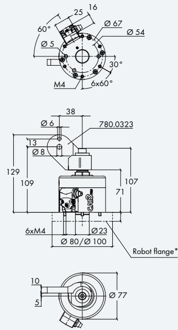
\* Flange thickness 10 mm or 15 mm depending on robot.
