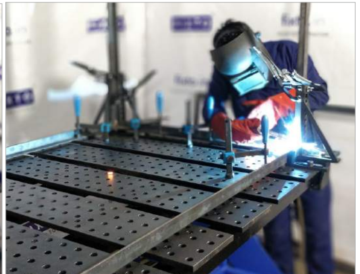
Welding in flat position
