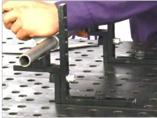
BLBAUTO can lock clamp to clamp and also plate to clamp
