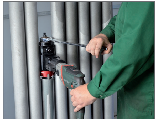
Minimum distance between tubes is 75 mm (2.95")
