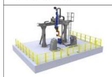
F10: Gantry head-tail 10-axis robot workstation Effective bear load: 2.5/5/10t
