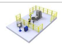
F2: Single station L shape 8-axis robot workstation Effective bear load: 1/2.5/5t
