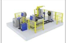
F3: Dual station head-tail type 8-axis robot workstation Effective bear load: 0.5/1/2.5/5t
