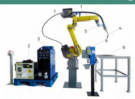
**Anti-collision Sensor:** When torch is colliding with other bodies, the anti-collision sensor will automatically send out collision-protection signal to robot, so as to protect robot and welding torch.
