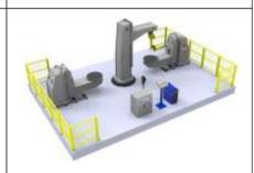
F6: Dual station rotation and lifting 12-axis hang upside down type robot workstation Effective bear load: 1/2.5/5t
