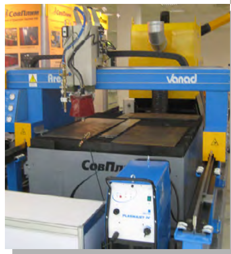
Sectional exhaust table CCT view 2
