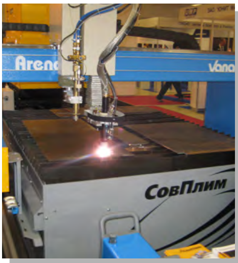
Sectional exhaust table CCT view 1
