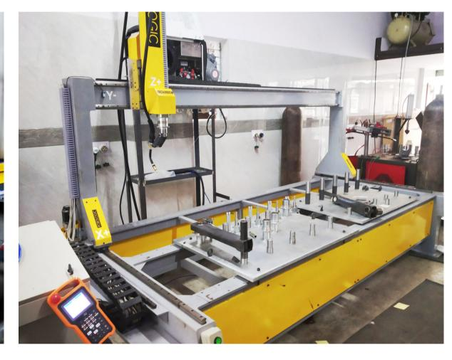
WELDING SCALE FRAME WELDING
