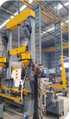
Elektra Vac Flux Recovery System have proven themselves as the most essential accessory to the entire Submerged Arc Welding process. They save value of flux, helps make better welds and produce all important saving in man hours. Flux Recovery unit keep abrasive flux away from moving parts on the welding ring. These systems are capable of separating out slag and fine flux returning only the clean reusable flux to the hopper.
