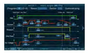
Adjustable welding parameters interface
