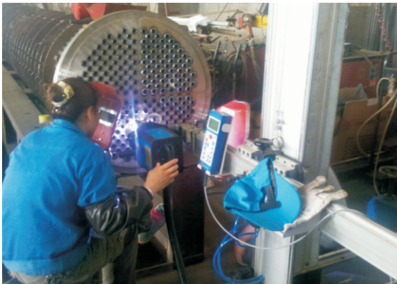
Heat exchanger in chemical industry Carbon Steel, 25mm 2 pass with wire feeding 1 Min per pipe
