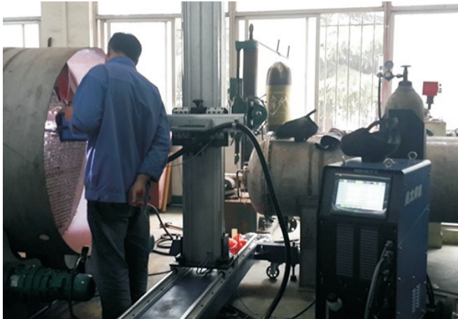
Wuhan, Hubei, China Stainless Steel, 15.5mm 1 pass No wire feeding 30 seconds per pipe
