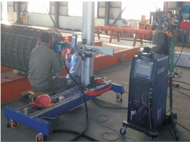
Dezhou, Shandong, China Stainless Steel, 25mm 1 pass with wire feeding 36 seconds per pipe
